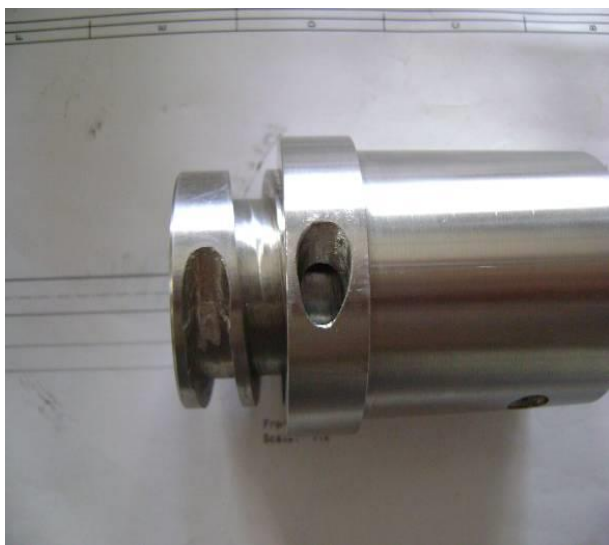
Fig. 1 Prototype made of micro room, outer mantle and regenerative body.
