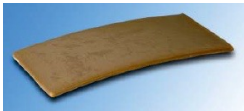
Demonstrator sandwich panel made of flax fiber reinforced top layers and flame retardants (A380 hat rack, scale 1:2)
