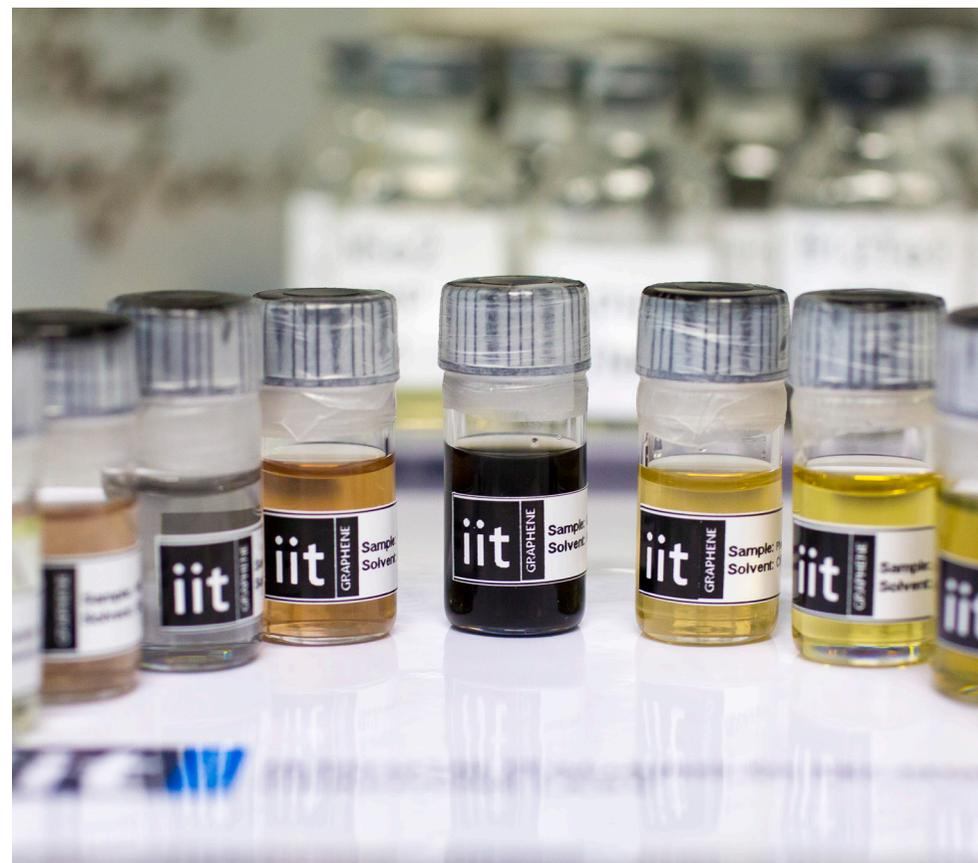
Figure 13: A selection of 2D-crystal-based inks developed by IIT.
